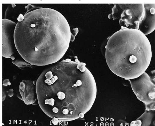
Fig. 2. Scanning electron photomicrographs of acid/alcohol treated (2% HCl/BuOH, 10 h) normal (a), high amylose (b), zero amylose waxy (c) barley starches.
